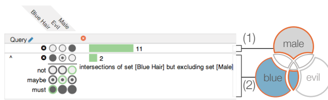
Fig. 9. The intersection query interface, defining a query for Simpsons characters that are either exclusively male or that have blue hair and aren't male . (1) The first logical OR clause requesting exclusive male characters is collapsed. (2) The second OR clause is shown in edit mode. The analysts can define whether a set must ●, may ● or must not ● participate in the queried intersections.
