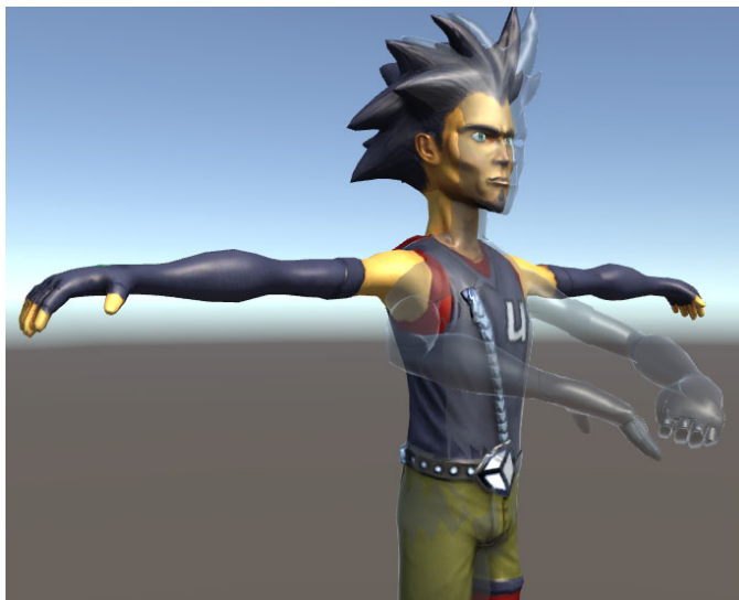
Fig. 5. An opaque avatar shows the actual pose, while a transparent target avatar depicts the target pose, which is to be taken. Image from [3].
