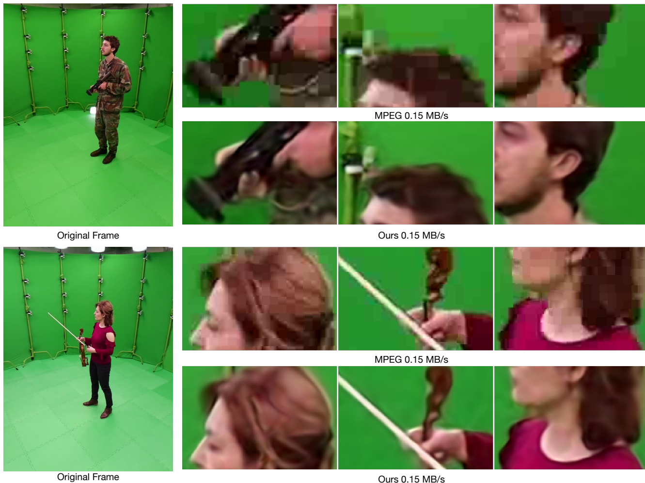
Fig. 5: Results on Dynamic Volumetric Light Field scenes. For each example frame, we show zoomed-in comparisons between MPEG (top) and our method (bottom). At a similar bitrate level, our method avoids the blocking artifacts commonly seen in MPEG-compressed content.
