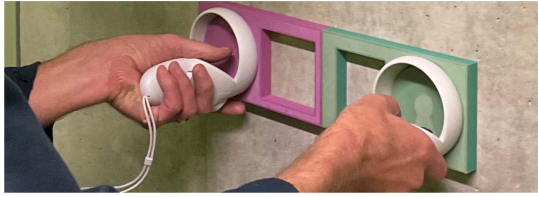
Fig. 3. 3D printed calibration station for controllers. Modular design allows printing left ( here: purple ) and right ( here: green ) elements with different socket orientations, thereby creating various configurations that facilitate distinctive identification features for each individual station.
