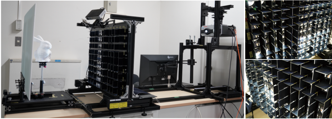
Fig. 7: The left picture shows the entire configuration of the developed system. The right shows close-up pictures of the kaleidoscopic array. The light-absorbing sheet was attached to the back side of each mirror against stray light.
