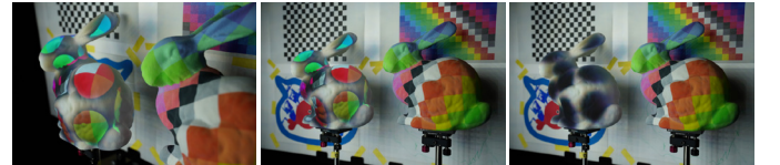
Fig. 13: Polka-dot PM using the proposed method was applied to the left bunny. The right picture shows the scene when the projector for PM was turned off.
