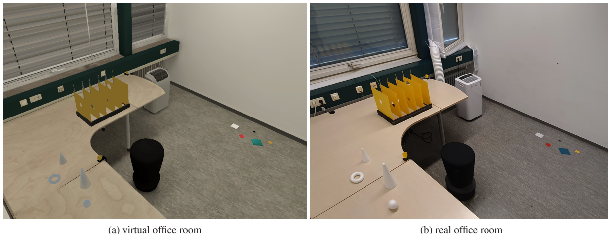
Fig. 1: Digital twin (a) of a real office room (b) used in the comparison of depth perception between VR and VST AR. The participants are seated on the stool and perform different depth-dependent tasks. Several objects (e.g., the cones, sphere, and ring on the table or the markers on the floor) are placed at various locations where the individual tasks are performed.
