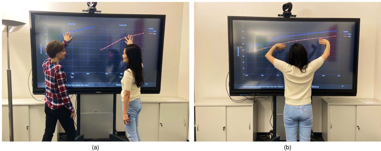
Fig. 5. Collaborative synonyms proposed for merging and splitting views. (a) Two participants perform two gestures to merge the views together. (b) One participant performs the gesture alone to split the view back into two.
