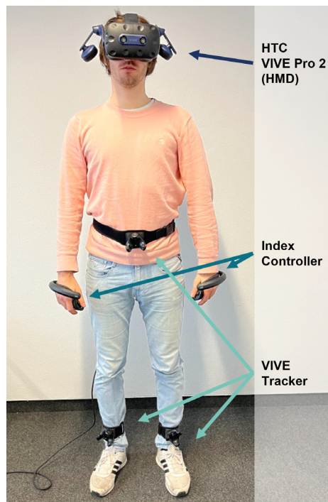
Fig. 4: Participants were wearing a HMD, Valve Index controllers, and three Vive Trackers, worn on the pelvis and each lower shin.
