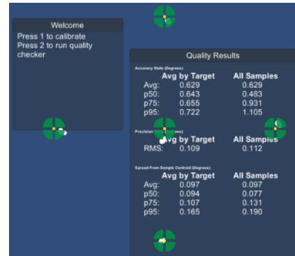
Fig. 2: Eye calibration quality utility, showing typical results, ran before each eye tracking block. Eye calibration keyboard button presses are managed by the experimenter.
