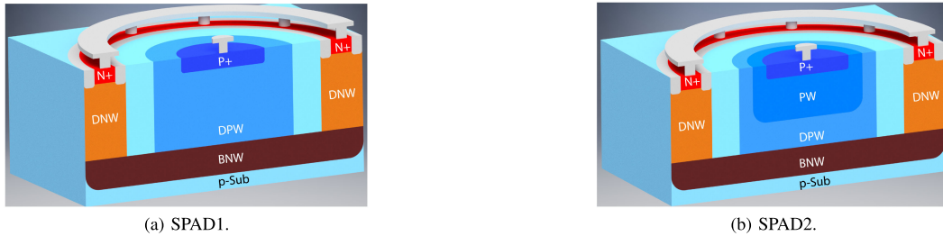
Fig. 1. Cross-sections of proposed 55 nm BCD SPADs. A single implant (PW) highlights the difference between structures.
