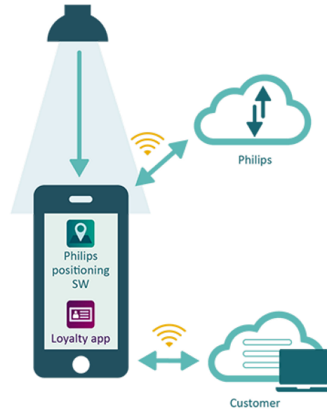
Fig. 6. Autonomous lamps emit unique codes. These are picked up by the phone camera. An Internet link (Wi-Fi 5 G,...) to a Signify - Philips data base allows the phone app to translate received codes and camera-measured angles into positions. A customer can use these data in a proprietary application.
