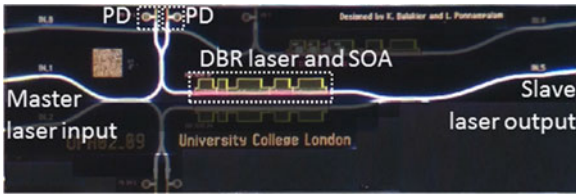
Fig. 9. Photographs of OPLL PIC with dimensions of 2 mm \times 6 mm. All components that do not form part of the OPLL are greyed out.
