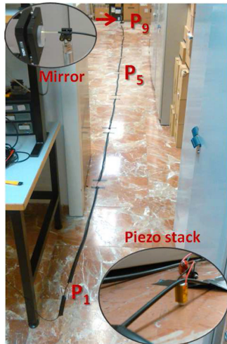
Fig. 3. Experimental set-up of the remote system for micro-vibrations detection. The sensing fiber is a standard SI-POF fiber of 11m-long with a 2.2 mm jacket directly attached to the floor. A piezoelectric stack is used to emulate periodic perturbations with amplitudes ranging from 1 to 6 \mu\text{m} at points P_1 , P_5 and P_9 , respectively.
