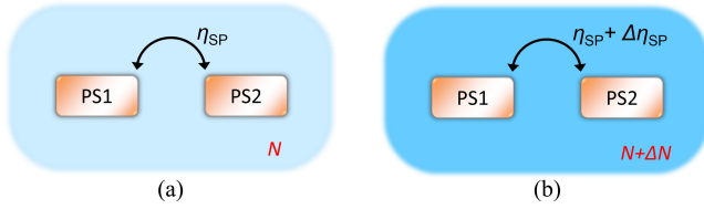
Fig. 3. Control of coupling efficiency via surface plasmon based on refractive index change of surrounding media. (a) Initial state and (b) active state.
