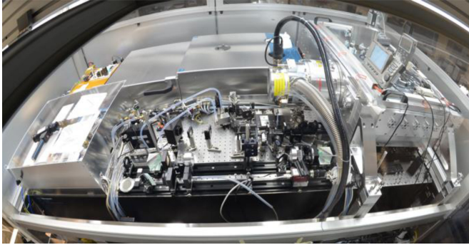
Fig. 18. Housed 2-stage Innoslab MOPA of Fig. 17 including spatial filtering, pulse-compression (front) and vacuum-chamber for experiments (right).
