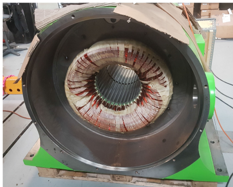
Fig. 11. Manufactured prototype stator.
