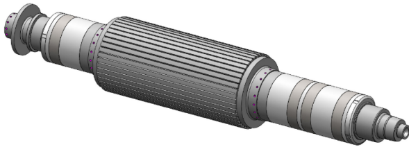
Fig. 4. Design of the rotor construction. Axially slitted solid rotor and three radial AMBs and one axial AMB.
