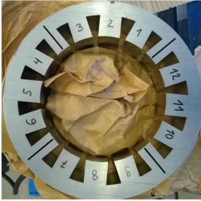
Fig. 8. Manufactured stator of E-core 12-pole radial AMB with flux barriers before the windings are installed.
