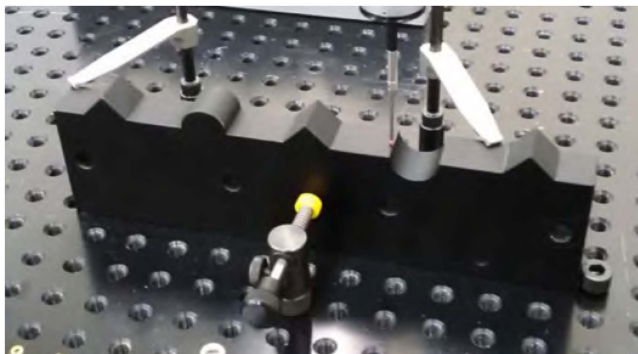
Fig. 13. Test piece during measurement in the coordinate measuring machine.
