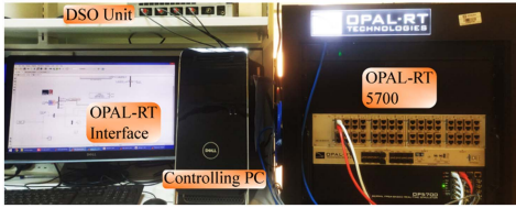
Fig. 17. OPAL-RT based HIL test setup.
