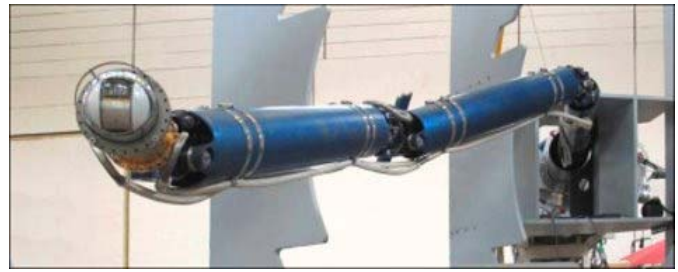
Fig. 6. WEST AIA in mock-up test.
