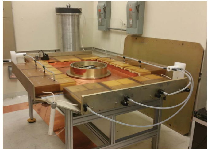
Fig. 32. Photograph of the 200-kA, 60-ns Lobo LTD at UNM in Albuquerque.
