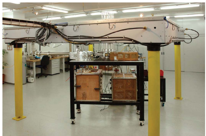
Fig. 29. Photograph of the 500-kA, 500-ns LTD at the Weizmann Institute of Science in Israel.
