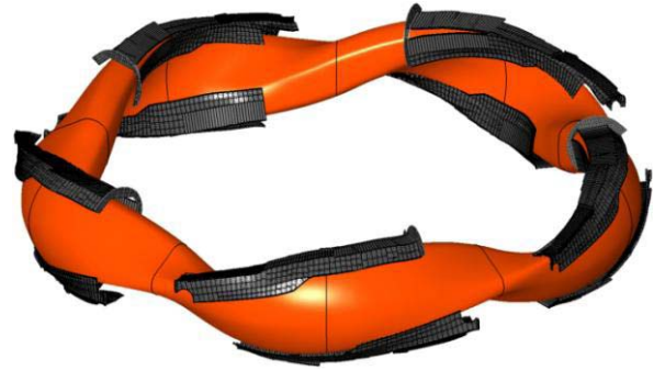
Fig. 2. (a) Plasma contour (orange) with five inboard limiters made of graphite (black stripes) defining the last closed flux surface. (b) Ten divertor units with the target plates following the topology of the resonant magnetic island divertor.
