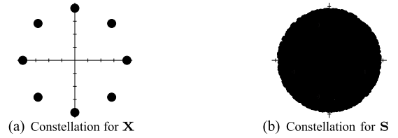
Fig. 6. Constellation diagrams for DSTBC [20] signals in \mathbf{X} and \mathbf{S} of (26), where M = 2 TAs and 8PSK are used.
