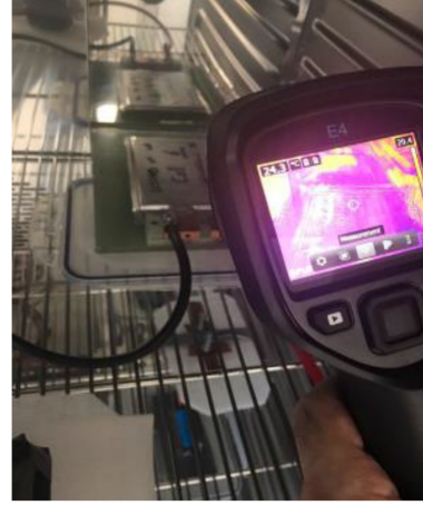
Fig. 7. Thermal camera used for checking cell’s surface temperature during the tests.
