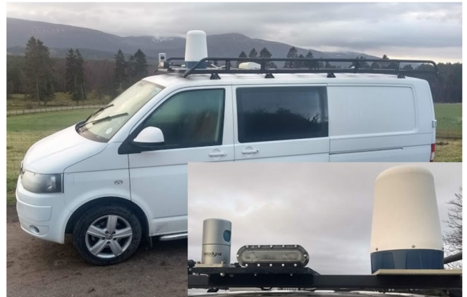
Fig. 1. The sensor suite and the test vehicle. This includes from left to right (Inset), a Velodyne HDL-32E LiDAR a Zed Stereo Camera pair and a Navtech-CIR104 79 GHz radar system.
