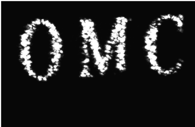
Fig. 5. CCD camera image generated by SLM.
