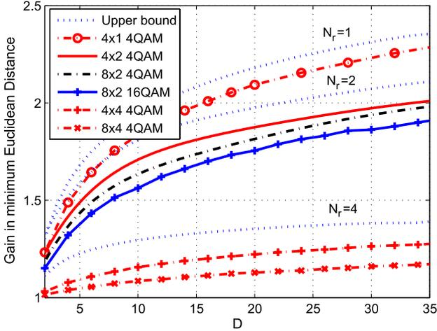
Fig. 3. Gain  $G$  in average MED for SM-CR with respect to SM for increasing  $D$ .
