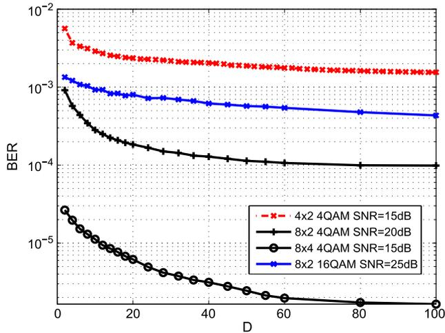
Fig. 8. BER versus  $D$  for a  $(4 \times 2)$ ,  $(8 \times 2)$ , and  $(8 \times 4)$  MIMO with SM-CR for 4QAM and 16QAM.
