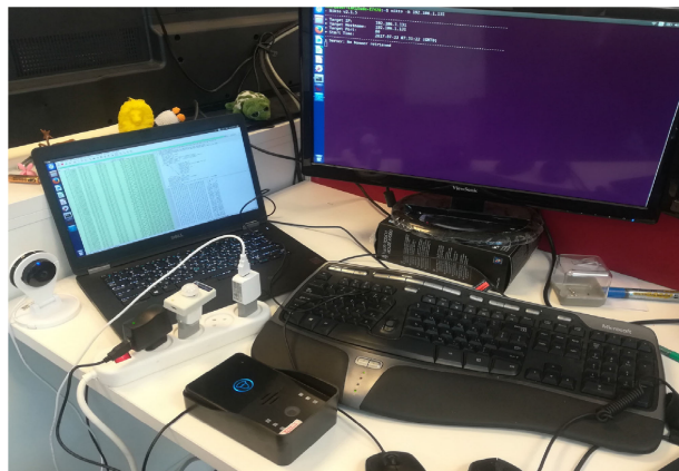
Fig. 9. Fuzzing setup environment in the security testbed.
