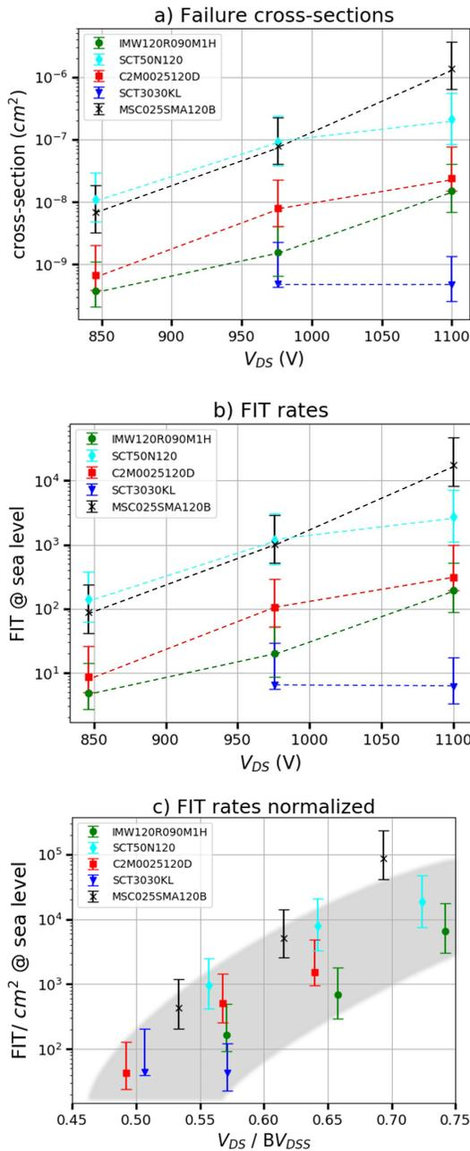
Fig. 5. (a) Failure cross sections of SiC MOSFETs from different suppliers as a function of the bias during the terrestrial neutron irradiations. (b) FIT rates for  $10^9$  h of operation. (c) FIT rates scaled by avalanche voltage and normalized with the active area.
