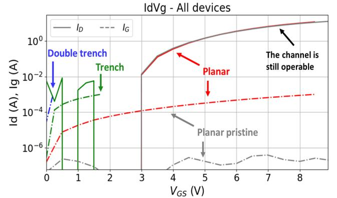
Fig. 7.  $I_D$ – $V_{GS}$  and  $I_G$ – $V_{GS}$  measurements performed at  $V_{DS} = 1V$ . The gate oxide is still operable for the planar Cree/Wolfspeed device (C2M0025120D) and the channel is still controlled by the gate voltage. Conversely, the gate oxide is heavily damaged and not operable anymore for the trench and double-trench structures.
