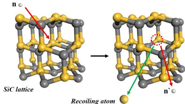
Fig. 1. By the elastic and inelastic scattering with the 4H-SiC lattice, the atmospheric neutrons produce recoiling atoms (i.e.,  $\alpha$ , C, Si, Mg, and Al) which generate ionizing tracks inside the power MOSFET.
