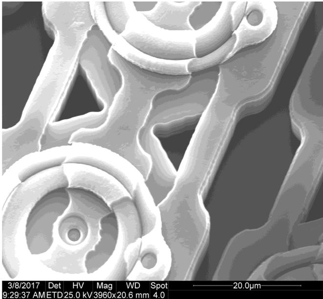
Fig. 12. Scanning electron microscope image showing a part of a sensor after excess silicon outside the SV was removed using plasma etching.
