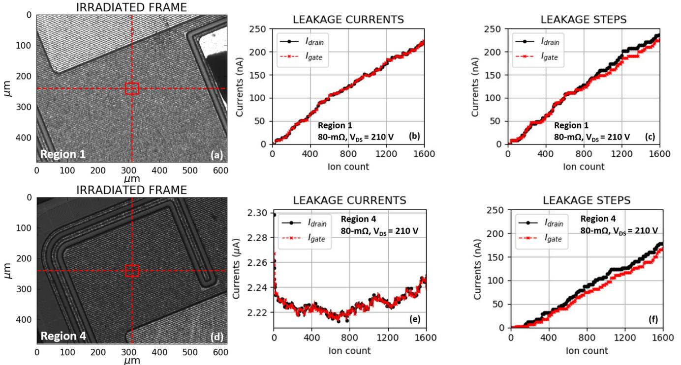
Fig. 2. Au irradiation in regions 1 and 4 of an 80-m $\Omega$  at  $V_{DS\ irr} = 210$  V. The exact location of the irradiation is identified by the window frame on the microscope images, respectively, in (a) and (d). The drain and gate leakage current increases are shown in (b) and (e) (for a pristine device, the leakage currents are on the order of 10 pA), while in (c) and (f) is the cumulative sum of the radiation-induced leakage steps.
