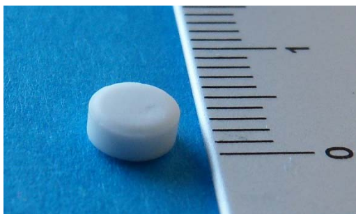
Fig. 20. Alanine dosimeter samples shaped in form of pellets [13].
