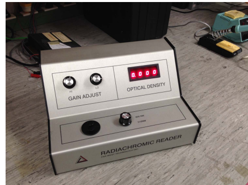
Fig. 11. Dual-wavelength photometer for readout of the FWT radiochromic dosimeters. The LED digital display reads directly in OD. The two wavelengths are 510 and 600 nm and are used to cover the range of the radiochromic dosimeters.
