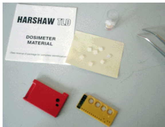
Fig. 13. TLD chips (bottom); the standard holder hosting the TLD chips during their readout.
