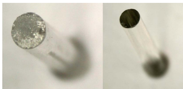
Fig. 22. Comparison of the top surface of a damaged crystal (left) versus an intact crystal with a smooth surface (right) [64].
