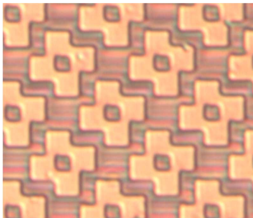
Fig. 10. SRAM back end of line and metal fill under 100X magnification.
