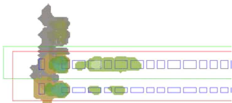
Fig. 7. Cross-section maps for the traditional DICE2 for states 0 and 1 (blanket patterns, master latch). The figure shows the maps for three different incidence directions, and three different LET values.
