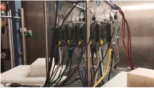
Fig. 2: Setup of the experiments showing the six irradiated Jetson-Nano boards.
