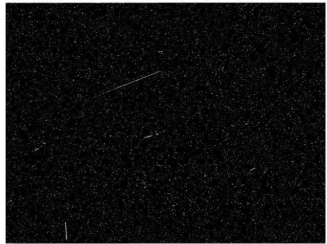
Fig. 5. CMOS imager under high proton flux irradiation
