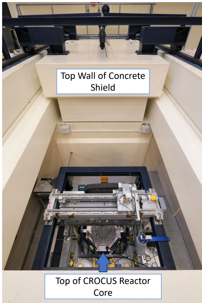
Fig. 2: Top-down view of the CROCUS reactor from above the concrete shield. The top wall may be opened when the reactor is shut down.
