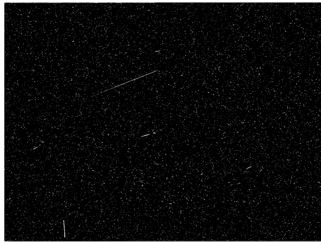
Fig. 5. CMOS imager under high proton flux irradiation.
