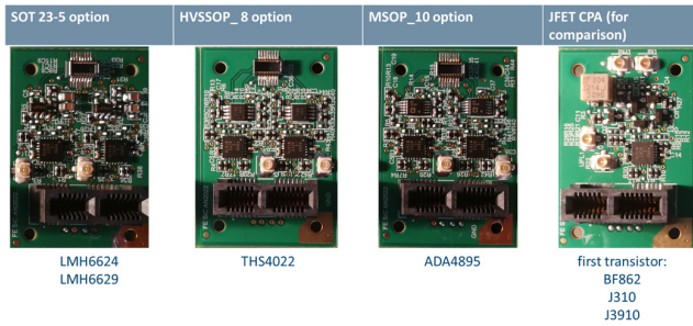
Fig. 5. Photograph of different four-channels charge preamplifier boards that have been produced (only the JFET design is a single-channel version).
