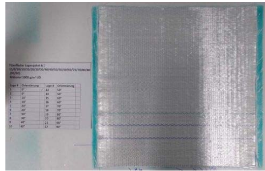
Fig. 20. Test sample of fiber layers with fiber orientations 2 \times 0^\circ , 2 \times 10^\circ , ..., 2 \times 90^\circ .
