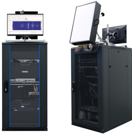
Fig. 7. Photograph of the realized demonstrator in a mobile rack, comprising the RF front end (black enclosure) on a steerable mount opposite the user interface, custom IF interfacing hardware, a standard personal computer, and a commercial dc power supply unit (PSU).
