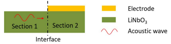
Fig. 7. 2-D model of acoustic wave propagating in a LiNbO 3 plate with and without top electrodes.
