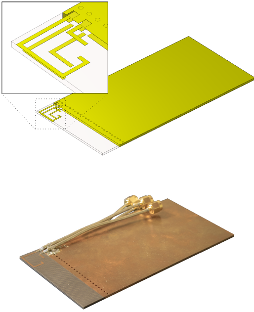
Fig. 2. Antenna used in this work consists of four antenna elements [29].
