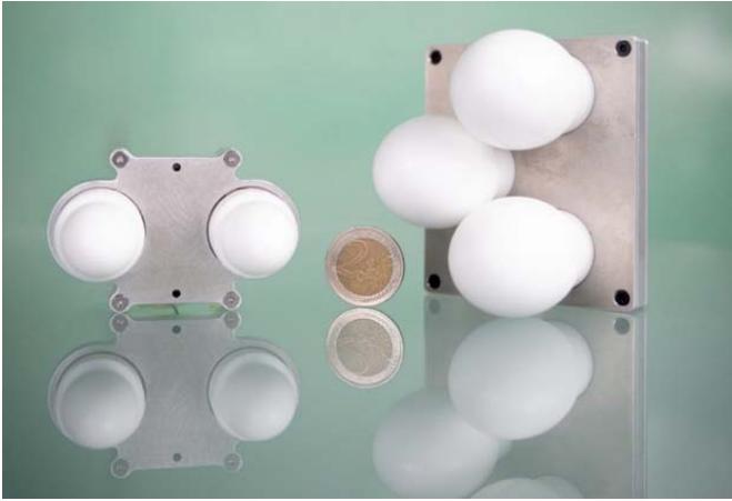
Fig. 1. Photograph of the dual-receiver 94-GHz radar system (right) with high output power and high bandwidth for high detection range and a small form factor realization with one transmitter- and one receiver-channel (left).
