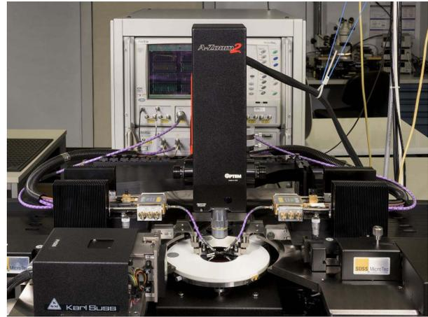
Fig. 6. PTB on-wafer measurement setup.
