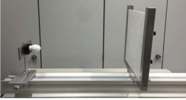
Fig. 2. Photograph of the measurement setup showing the radar sensor on the left-hand side and the sample holder on the right-hand side on an optical rail.
