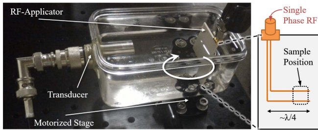
Fig. 8. Circular scanning of a bulky, off-the-shelf transducer using a motorized stage, together with a simple dipole RF applicator, can result in high-resolution TA cross-sectional images [47].
