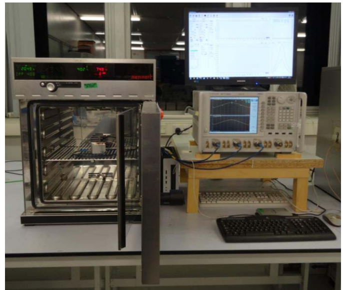
Fig. 6. Photograph the bench-top experimental assembly. The Sensor is put inside a computer-controlled oven and connected to an Agilent PNA-L N5232A network analyzer under LabVIEW program control.
