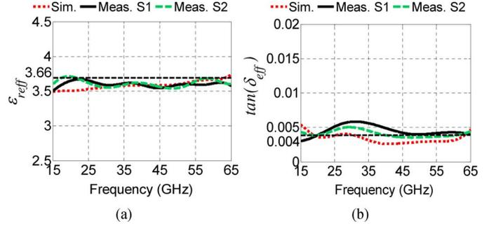
Fig. 5. Measured and simulated: (a)  $\epsilon_{\text{reff}}$  and (b)  $\tan(\delta_{\text{eff}})$  of the delay section for two fabricated sets of the (1-mm long) line standard.
