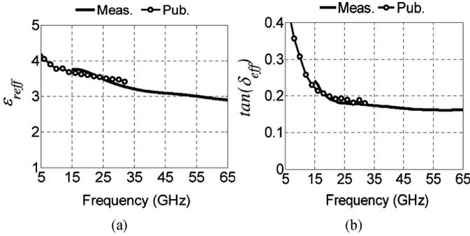
Fig. 7. (a) Dielectric constant and (b) loss tangent of LC cell containing Isopropanol; Pub. data from [31] and Meas. data from this work.
