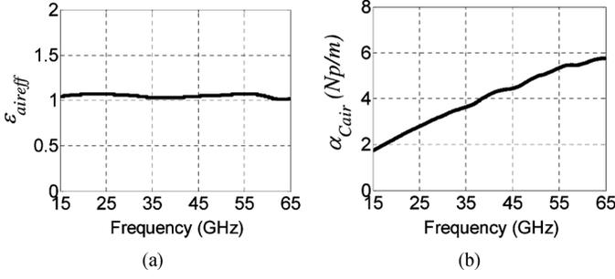
Fig. 6. (a) Dielectric constant and (b) attenuation constant due to conductors of the air-filled LC cell.
