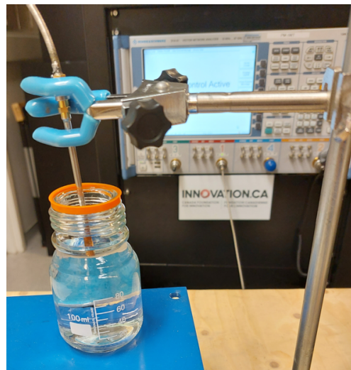
Fig. 6. Extracting dielectric spectrum of the calibration liquids using a commercial dielectric probe: an open mode probe method dielectric constant and dielectric loss tangent measurement system, DPS16, from KEYCOM Characteristic Technologies through a ZVA 67 VNA from Rohde&Schwarz© from 0.5 to 6 GHz.
