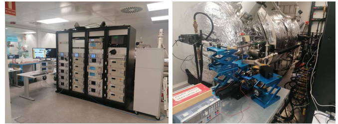
Fig. 5. Assembled PIM setup based on the multicarrier facility for the enhanced multicarrier scenario.
